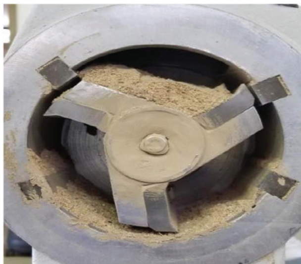
Fig. 4. Grinding chamber after grinding. Grinding leftovers represents the plugging of the screen.
