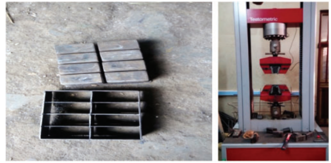
Fig. 1. (L-R) Fabricated mould for snack bar shaping. Testometric materials testing machine.
