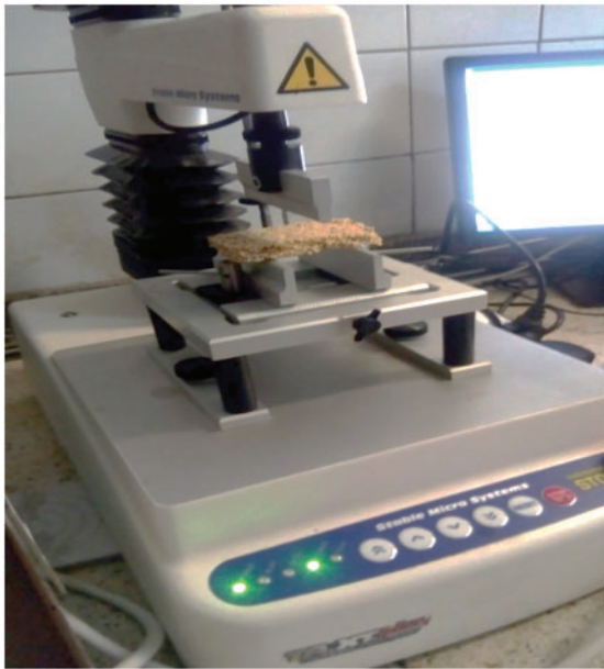
Fig. 2. Hardness analysis of snack bar samples.
